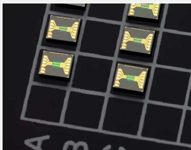
Axetris mass flow sensor chip
