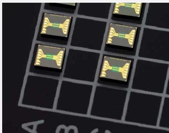
Axetris mass flow sensor chip
