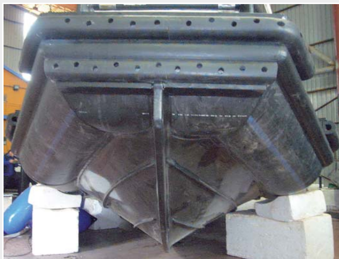
Boat underside with blunt-welded and extruded parts
