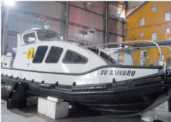
Fully-welded plastic boats made from PE for carrying passengers...
