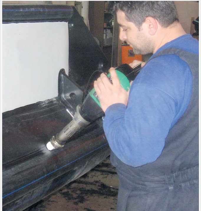
Extruding with the handy WELDPLAST S2
