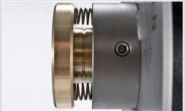
The tension brake disc ensures constant tension when rolling off the strap.
