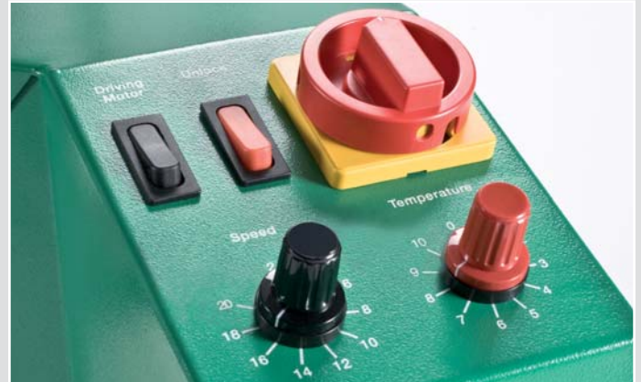
The well arranged operating unit offers simple control of the relevant welding parameters speed and temperature.
