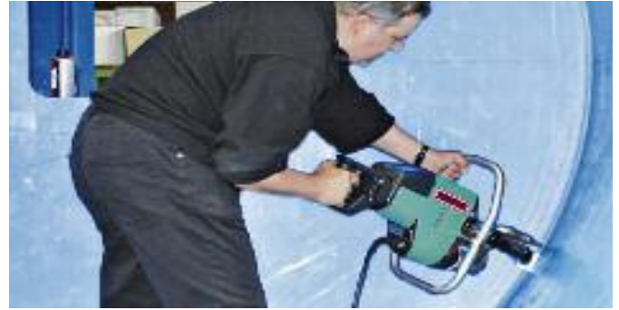
The WELDPLAST S6 is guided easily with the practical control wheel grip.
