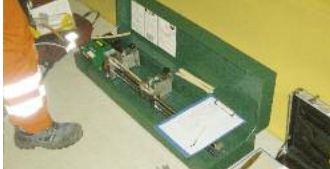
Seam tests can be conducted in the lab or on-site with the EXAMO USB.
