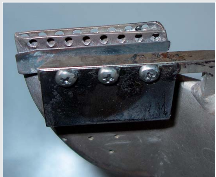
Upper part of grip-nozzle with (sheet pressure plate) downholder – the burls (grips) are hidden underneath.
