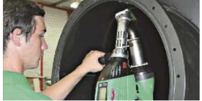
Even inside radiuses are easy to weld.
