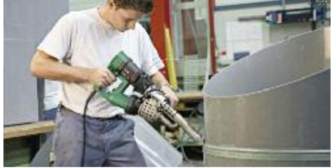
FUSION 3C during the welding of a V-seam.
