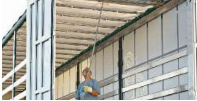
Tarpaulin bows for fixed and sliding rooftops of trucks. (picture: Krone)
